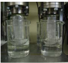
Melting ice core samples in the methane extraction line at OSU. Photo by Logan Mitchell
