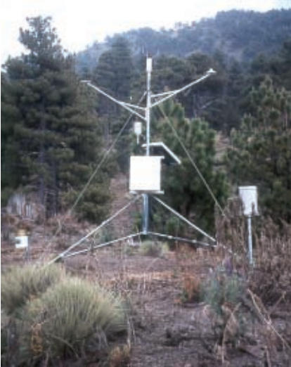
Figure 2. An automated weather station at 3760 m elevation on Nevado de Colima, Mexico, providing the climatic timeseries against which data on ring growth can be calibrated. [5] Photo: F. Biondi
