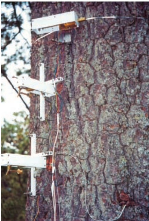
Figure 1 Instrumentation installed on a Pinus hartwegi tree to measure radial changes both above and below the bark as a means of better calibrating tree ring growth as a function of climate variables. [5] Photo: P.C. Har-sough
